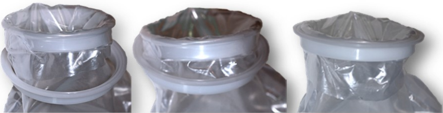
Photo Sequence Showing Ezi-Dock Docking Ring Attachment to Charge Bag Opening
